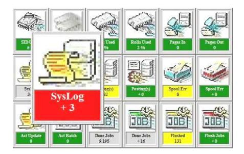
This example shows the behaviour of the object "SysLog". Used is the option "Zoom. By using the option "Keep" only the new messages are interpreted. In this sample a single object was selected by double click and is show as zoomed. The objects "Posting(s)", "Spool Err" and "Flush Jobs" no new values were present.
